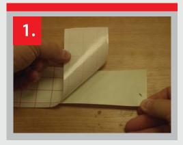
1. Peel backing strip off to expose the adhesive.
