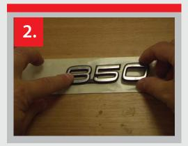
2. Place the badge onto the adhesive face. Apply pressure evenly onto the badge and on the back.
